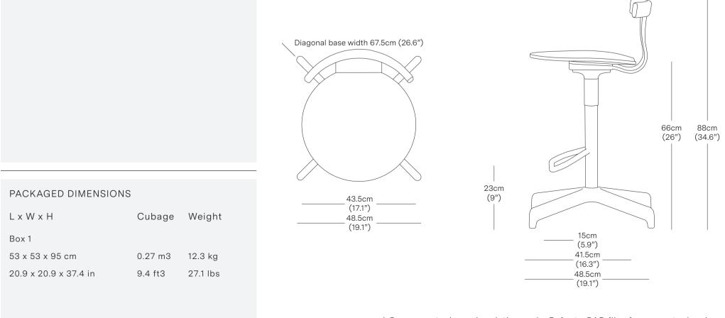
\* Components drawn in relative scale. Refer to CAD files for accurate drawings.
